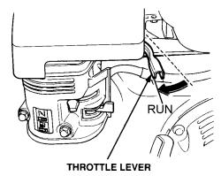
Figure 13. Throttle Lever (Run)
